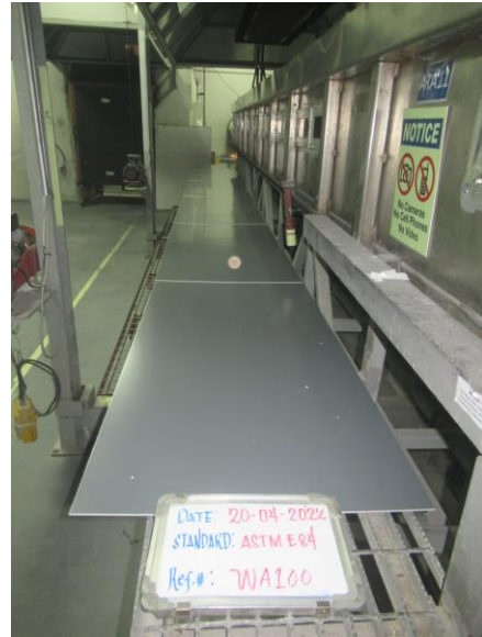
Photo 2: Specimen before the test. (Fire Side)
