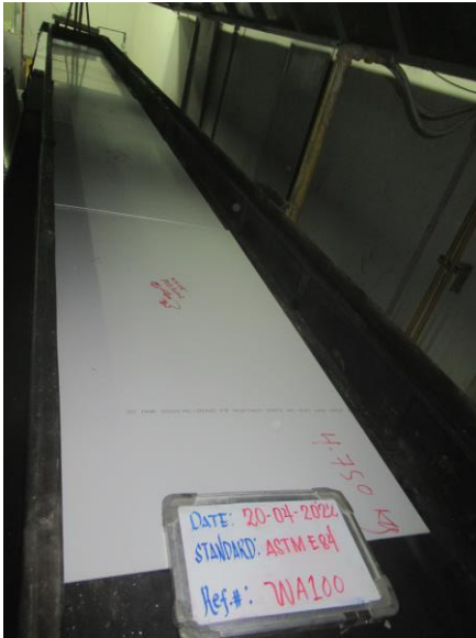
Photo 1: Specimen before the test. (Non-Fire Side)
