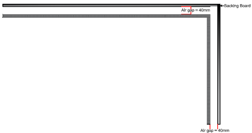
Drawing 2: Top view of the mounted specimen with airgap. All dimensions are in millimeters (mm).
